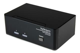
The SV231DD2DUA 2-port Dual DVI USB KVM Switch allows two PCs, each with dual DVI video outputs, to share two monitors, one microphone and set of speakers, one keyboard and one mouse as well as two other USB peripherals.
